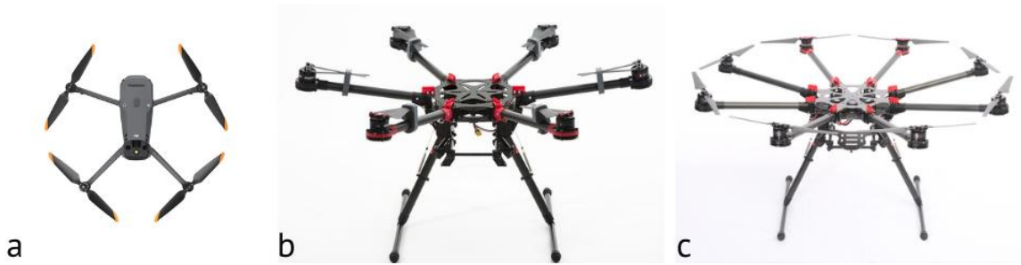
Şekil 11. a) Quadrotor, b) Hexacopter ve c) Octocopter
